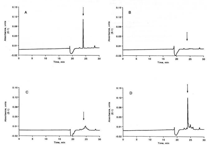
Fig. 3. Typical chromatograms (arrow indicates fenoxycarb): (A) - fenoxycarb standard 0.2  $\mu$ g/mL; (B) - reagent blank; (C) - 5 g untreated control apples; (D) - 5 g control apples fortified at 0.1 mg/kg (80.9% recovery).
