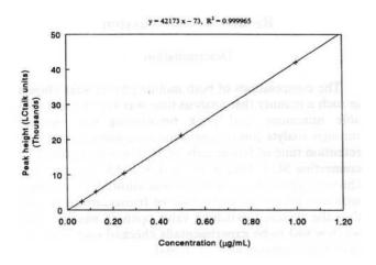
Fig. 2. Peak height calibration over concentration range 0.06 - 1.00 μg/mL for fenoxycarb.
