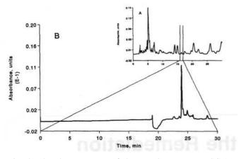
Fig. 4. The chromatogram of the sample extract on SC-1 clean-up column 1 coupled directly to UV-PDA detector (A) and the chromatogram of SC-1 effluent portion on SC-2 analytical column 2 (B). The fenoxycarb peak is identified by its retention time (24.1 min).
